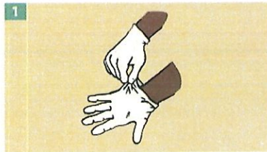
1 Grasp the outside of one glove at the wrist. Do not touch your bare skin.
